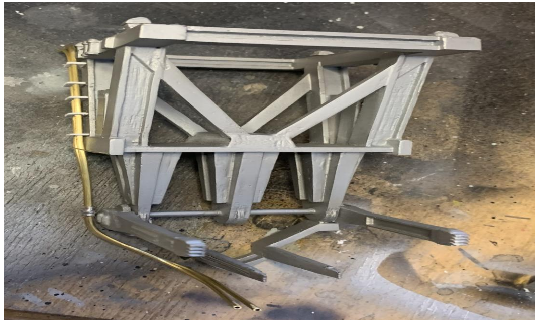
Launch Gantry in progress with brass tubing for wire conduits.
