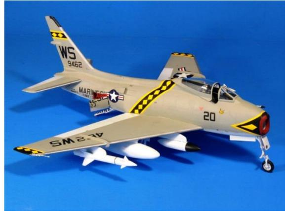
The original contract for 100 FJ-1 Furies was reduced to 30 production models. Next came the FJ-2 Fury which was basically a navalized F-86E Sabre. Changes included a tail hook and lengthening of the nose landing gear. After producing 200 FJ-2s the navy wanted improved performance and re-engined it with the Wright J65 Sapphire engine (License built British Armstrong Siddeley powerplant). 538 FJ-3s were built. Versions of the Westinghouse powerplant powered subsequent models of the Fury.
