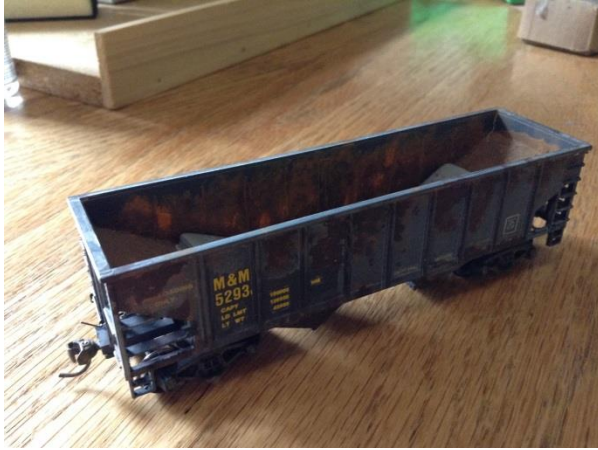
Paul Lessard Built this 50ton ballast car from Walther's. He added weights and uncoupling levers. He weathered it with chawks, custom paint blends, and washes.
